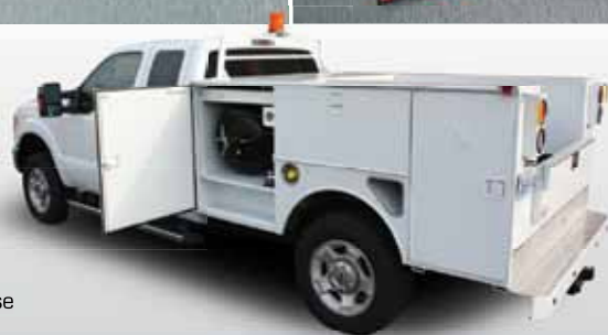
▲ S 96 ST Transverse Service Body housing CNG Tank
